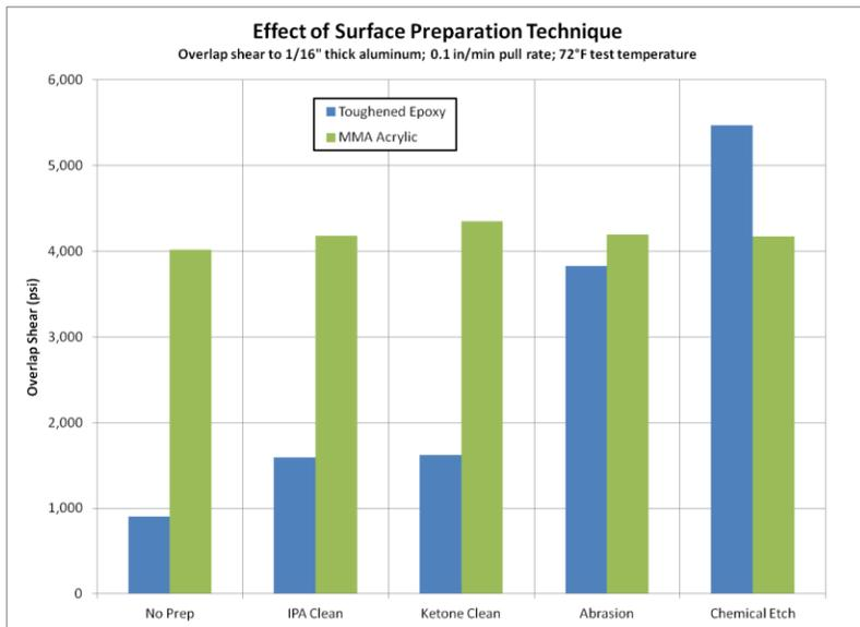
Figure 3: Effect of surface preparation on bond strength
