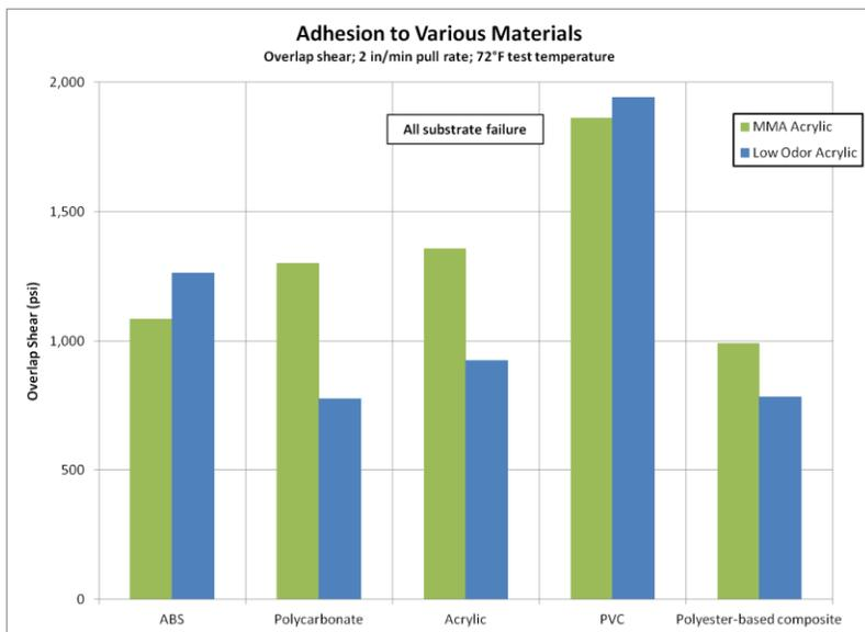
Figure 6: Bond strength to plastics and polyester-based composite
