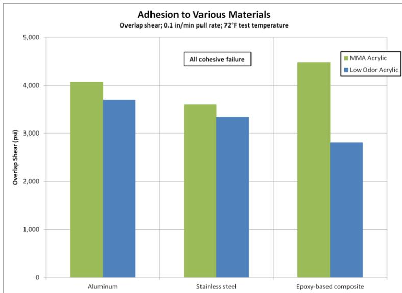
Figure 5: Bond strength to metals and epoxy-based composite
