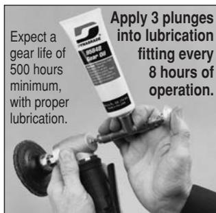
Expect a gear life of 500 hours minimum, with proper lubrication.
