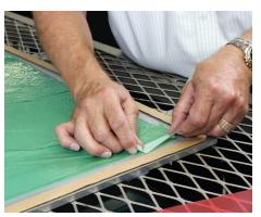
Works inside the bagging area to securely hold/position laminate plys, release liners, bagging materials and thermal couple wires while providing clean removal post cure.
