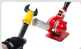
Apply a Heat Shrink Link over an attachment point that uses Quick Wrap Tape. Apply heat using a heat gun until the link shrinks completely. Do not burn the Heat Shrink Link.
